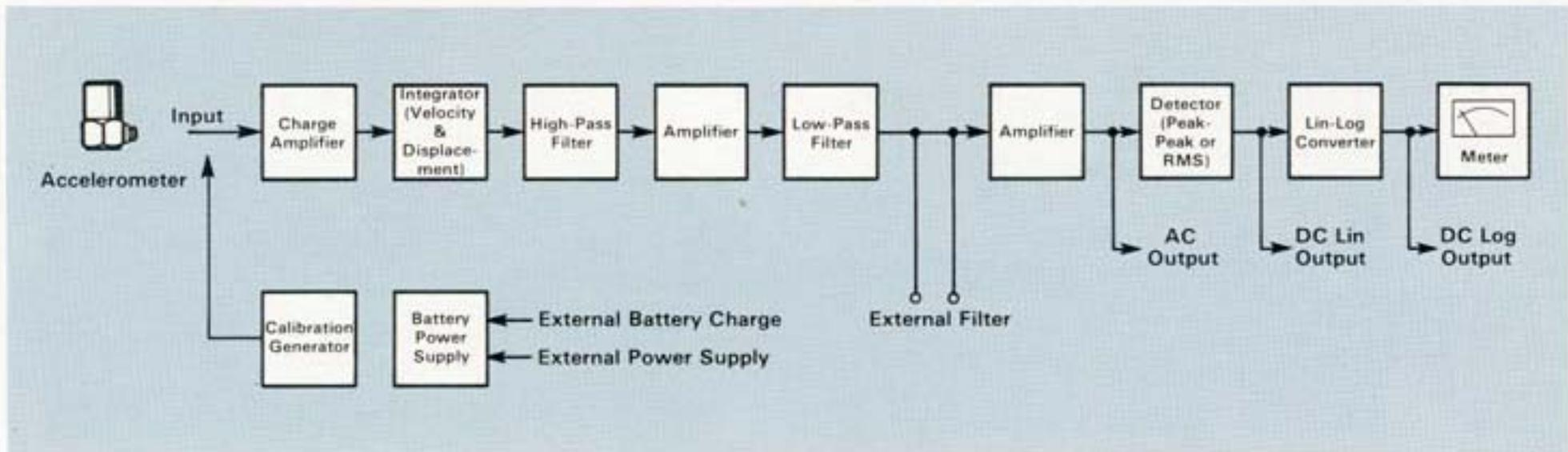
The block diagram shows how a typical modern vibration meter is built-up. The accelerometer is connected to a charge amplifier input stage with an input impedance of several  $G\Omega$  so that a separate preamplifier is not necessary. With a charge amplifier input, long input cables from the accelerometer, (up to several hundred meters), can be used without any appreciable loss in sensitivity.
