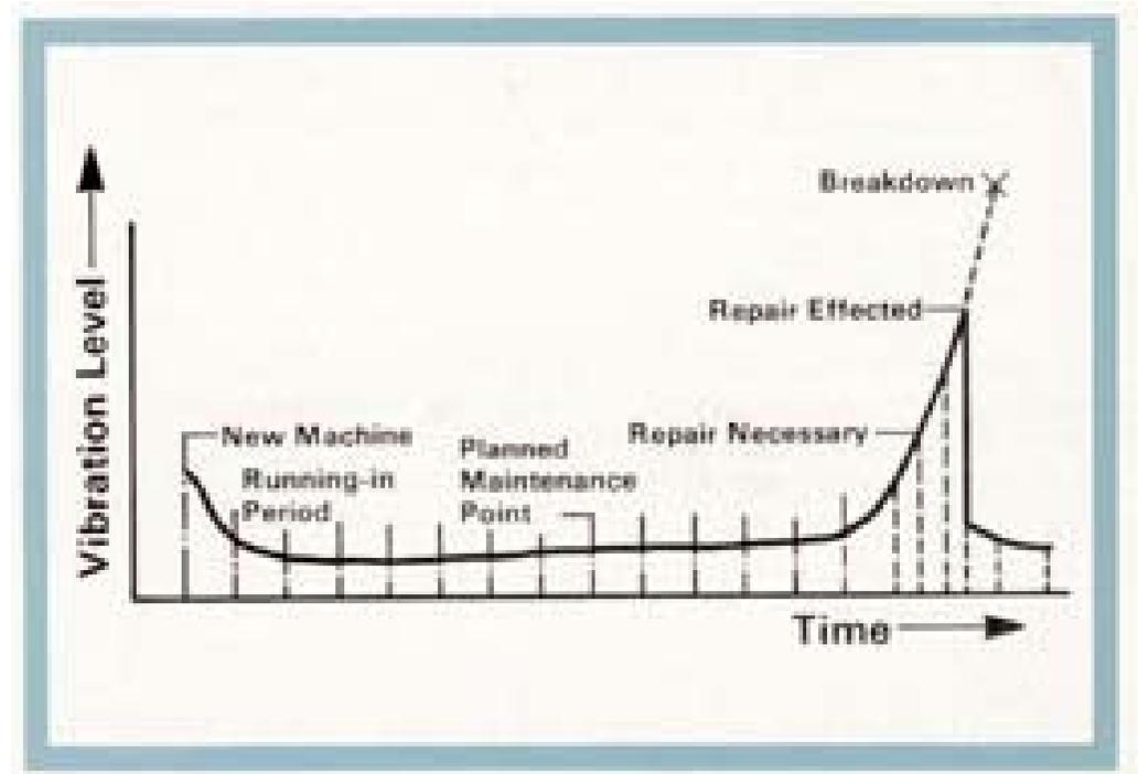
can therefore be used as a reference "signature" for that machine. Subsequent analyses can be compared to this reference so that not only the need for action is indicated but also the source of the fault is diagnosed.
